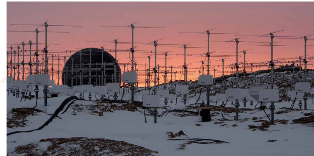
The large-scale PANSY (Program of the Antarctic Syowa MST/IS Radar) antenna array installed at the Syowa Station
